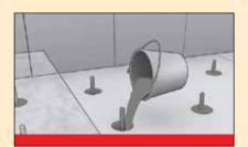
Use Ramco Super Grout -Epoxy to attach new reinforcement to the old slab.
