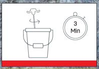
Stir for 3 minutes until smooth, then rest for 2 minutes. Stir again for 2 minutes before applying. (Do not add sand or other materials).
