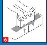
Place the next block over the coated surface and press it firmly
