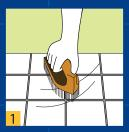
Clean thoroughly on the tile joints area. Remove all the loose materials, oil, grease and other impurities.
