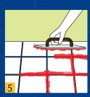
Fill the paste between tile joints within 1 hour of mixing and wait for 10 minutes for drying.
